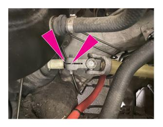
Please repeat this procedure several times in the 3–4 days before the repair; this makes it easier to loosen the connection between the steering gear and the steering column.
